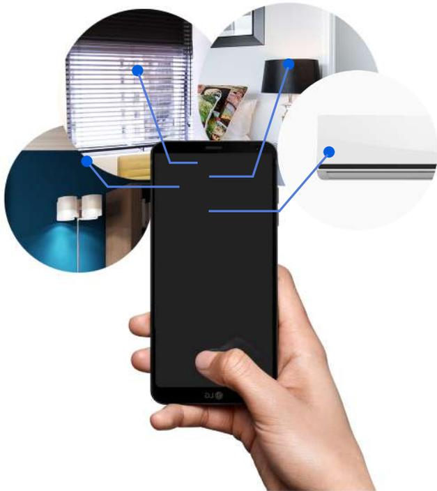
Caeigo Connect IoT engine has all the building blocks built in for controlling the smart enabled room controls installed within the hotel rooms. Caeigo Connect gateway that goes into the hotel rooms has the support for Zigbee, Z-Wave, Bluetooth LE and Wi-Fi protocol support to execute any control commands from the guests through the digital touchpoints offered by Caeigo Connect.
